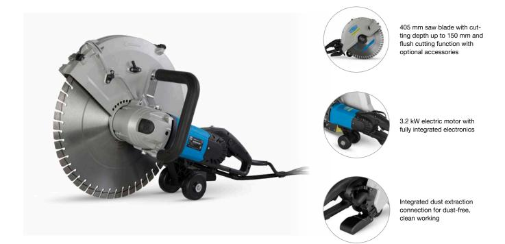
The HBE400 is a 3.2 kW hand-held saw for cutting depths up to 150 mm. In combination with our accessories kit, this hand-held saw is excellently suited to flush cutting. This model can be used for both wet and dry applications and its integrated dust extraction connection enables clean working. The compact design, low weight and detachable guide rollers guarantee ease of handling and machine guidance for the user. The 230 V electric drive enables flexible working indoors and outdoors.
